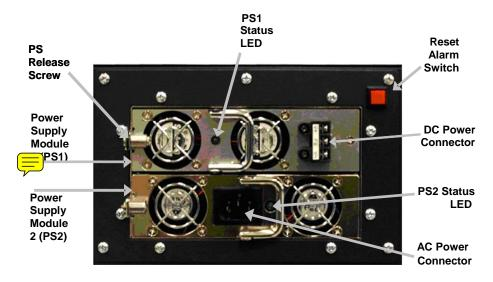
Redundant ACDC Power Supply, Close-Up
